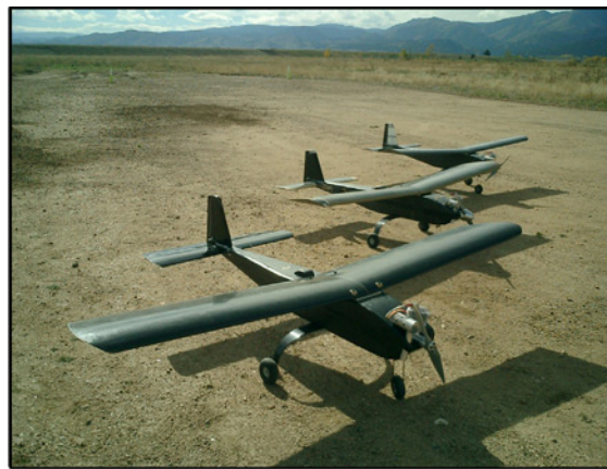
Fig. 8b Three Ares UAs on the ground at the local flight test facility.
